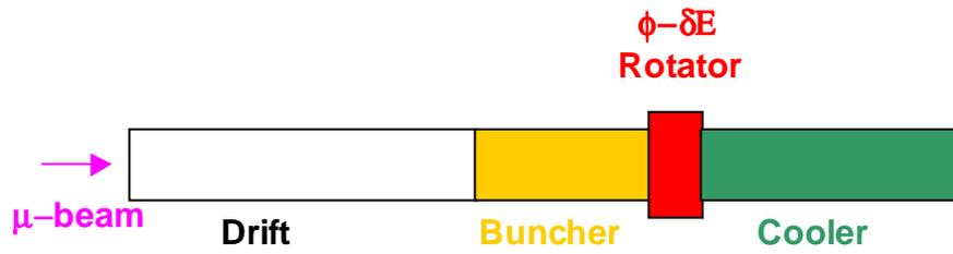
Fig.4 Overview of the transport system used above, which is a 100m drift, a 60m buncher, a 8.4m.  $\phi$ - $\delta E$  rotator, and a 100m cooling system.
