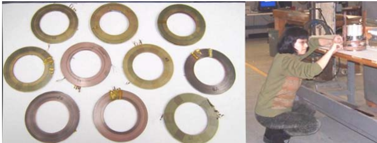
Fig. 11: Ten HTS pancake coils (see left) made with YBCO from SuperPower for the 20 T solenoid now under construction at BNL. The picture on the right shows a double-pancake coil being prepared for intermediate test.
