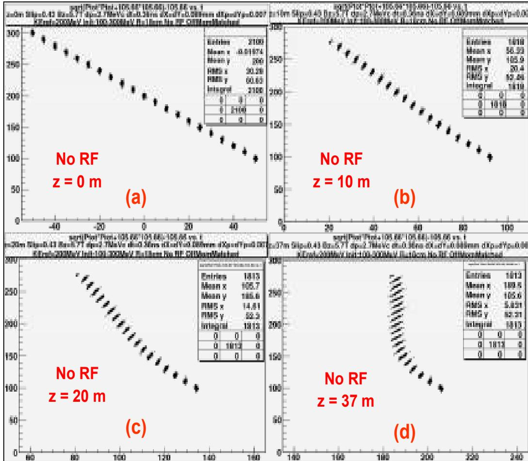
**Figure 5:** Kinetic energy (MeV) versus time (nsec) for muon bunches in the helical channel without RF at the start at  $z = 0$  m in (a),  $z = 10$  m in (b),  $z = 20$  m in (c), and end of channel at  $z = 37$  m in (d). Neighboring bunches are separated by 10 MeV and 5 nsec with energy range from 100 to 300 MeV.
