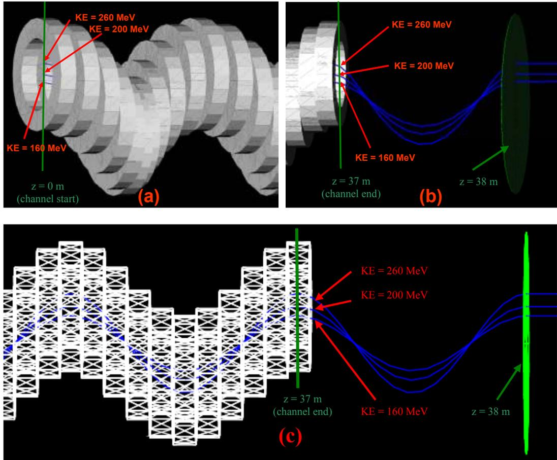
**Figure 4.** Display of muons with kinetic energies 160, 200, and 260 MeV that are momentum matched to the helical channel at the start in (a) and end in (b) and (c). Muon tracks past the end at  $z=37$  m are shown to better illustrate the trajectories and the green disk in (b) and (c) is placed at  $z = 38$  m, which is one period past the channel end; each muon travels a full helix period between  $z = 37$  m and 38 m.
