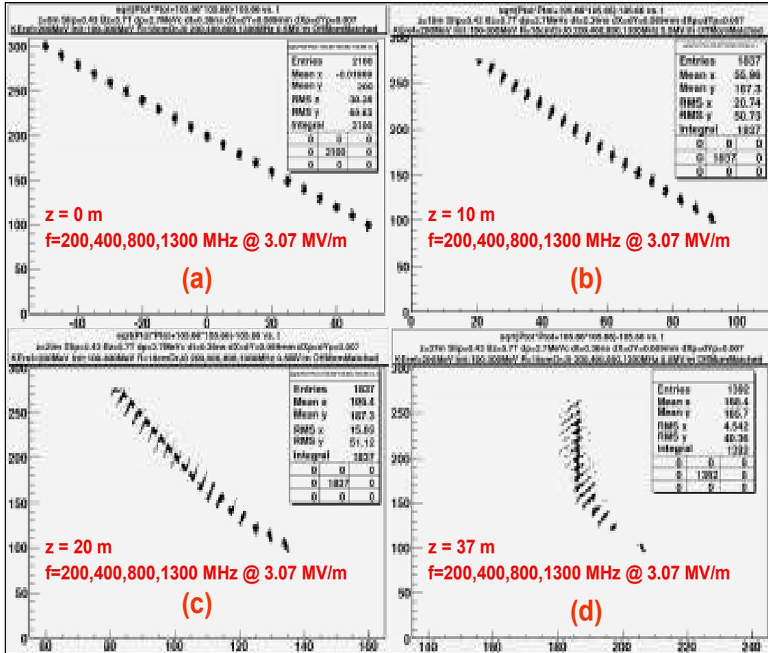
**Figure 9:** Kinetic energy (MeV) versus time (nsec) for muon bunches in the helical channel with RF where only discrete frequencies of 200, 400, 800, and 1300 MHz are used. KE vs. t at channel start at  $z = 0$  m in (a),  $z = 10$  m in (b),  $z = 20$  m in (c), and end of channel at  $z = 37$  m in (d).
