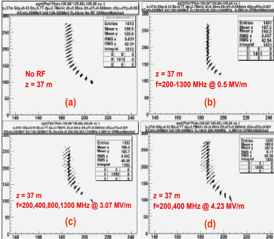
**Figure 11:** Kinetic energy (MeV) versus time (nsec) for muon bunches at the end of the helical channel without RF and the various RF schemes.
