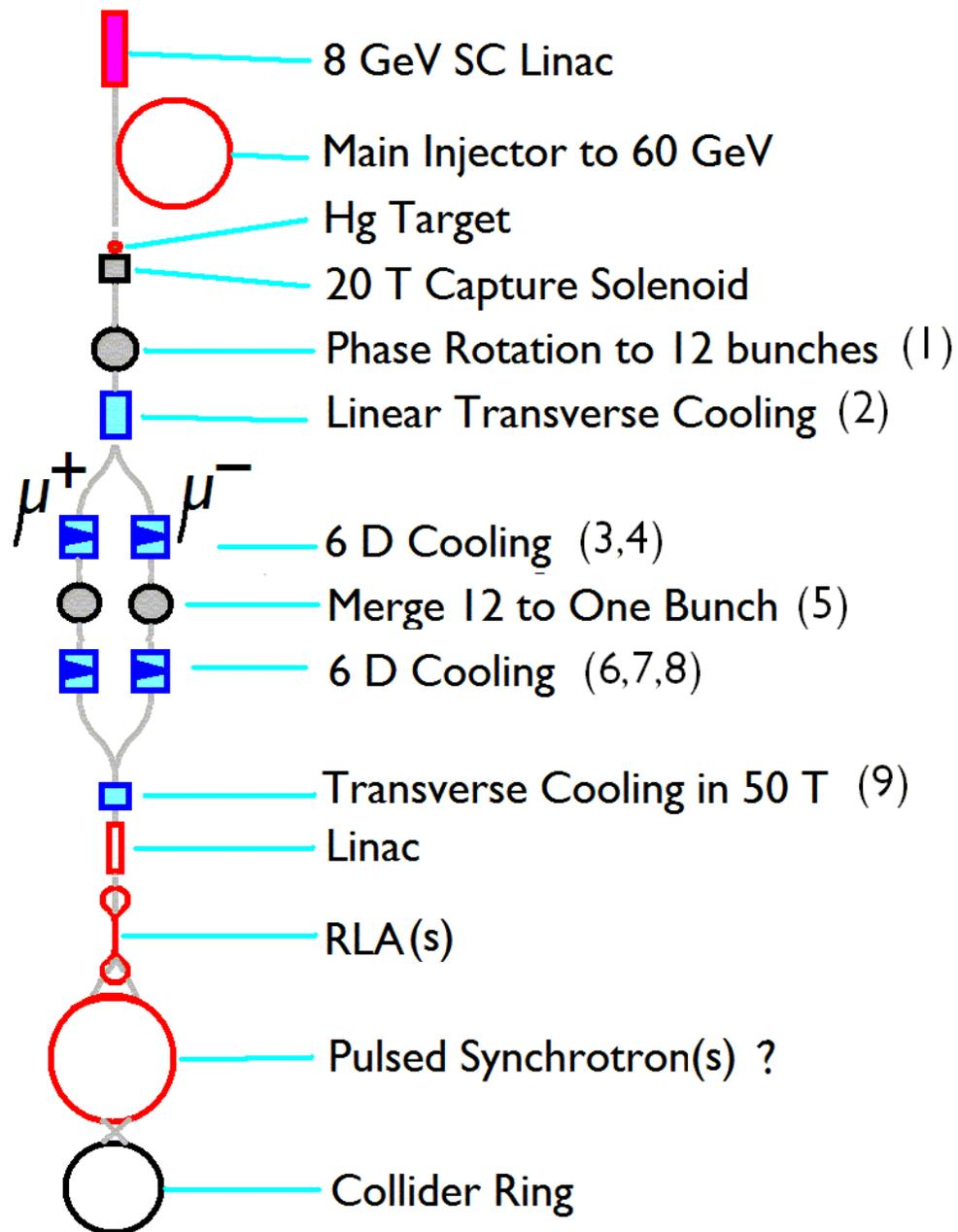
**Figure 1.** An overview of the muon collider system, showing the muon production, phase-energy rotation and cooling of 12 muon bunches, bunch recombination to 1 bunch, followed by more cooling and acceleration into a storage ring. [2]
