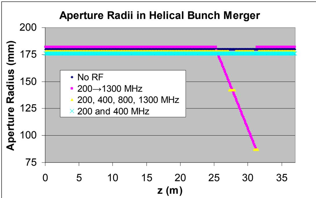
**Figure 7:** Aperture radii versus longitudinal position in the Helical Bunch Merger Channel for cases without RF as well as the RF schemes studied. Radii at 180 mm have been displaced for sake of clarity to elucidate the schemes which share that radius.
