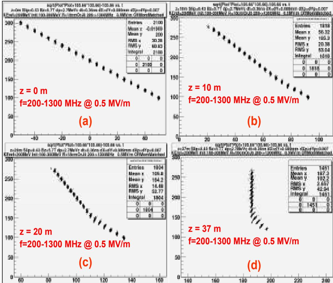
**Figure 8:** Kinetic energy (MeV) versus time (nsec) for muon bunches in the helical channel with RF where each cavity has frequency tuned for reference neighbors with frequencies between 200 to 1300 MHz. KE vs. t at channel start at  $z = 0$  m in (a),  $z = 10$  m in (b),  $z = 20$  m in (c), and end of channel at  $z = 37$  m in (d).
