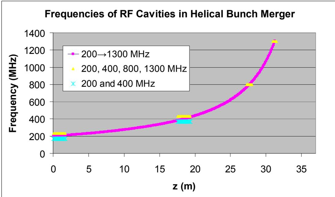
**Figure 6:** Frequencies of RF cavities versus longitudinal position in the Helical Bunch Merger Channel for the various RF schemes. Frequencies at 200 and 400 MHz have been displaced for sake of clarity for displaying other nearby frequencies.
