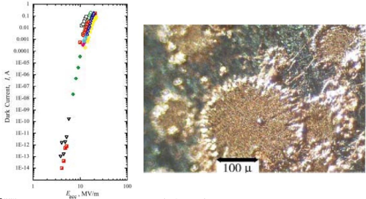
Figure 14: Dark current measurements in rf cavity in a magnetic field. Damage to the cavity can be seen.
