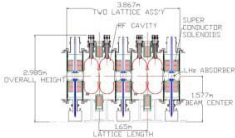
Figure 11: Two cells of the 1.65 m cooling lattice.
