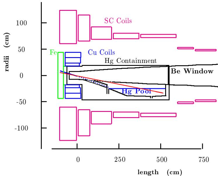
Figure 8: Target, capture solenoids and mercury containment.
