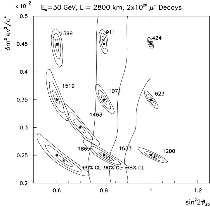
Figure 2: Fit to muon neutrino survival distribution for  $E_\mu = 30$  GeV and  $L = 2800$  km for 10 pairs of  $\sin^2 2\theta$ ,  $\delta m^2$  values. For each fit, the  $1\sigma$ ,  $2\sigma$  and  $3\sigma$  contours are shown. The generated points are indicated by the dark rectangles and the fitted values by stars. The SuperK 68%, 90%, and 99% confidence levels are superimposed. Each point is labelled by the predicted number of signal events for that point.
