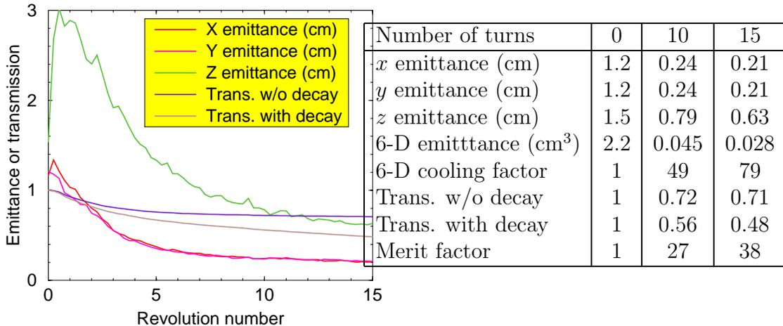
Figure 18: Evolution of the beam emittance/transmission at the TETRA ring cooler.
