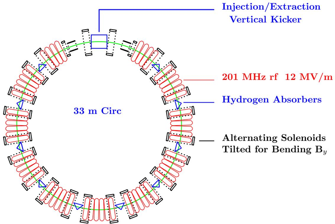
Figure 19: Layout of an RFOFO cooling ring.
